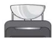
To remove the mouthpiece, simply pull directly upwards.
