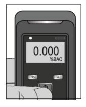
In NORMAL MODE operation a 3 decimal place result will appear on the display and remain for 15 seconds. eg. 0.051%BAC
