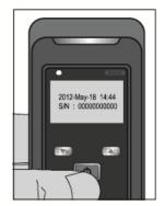
Depress the ON/OFF button for 2 seconds until the breathalyser turns on.
