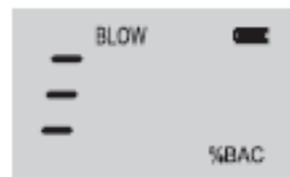
Once the correct amount of air is received the breathalyser will stop beeping and start analysing the sample. 3 dashes will circle around the screen while analysis is taking place and the word ANALYZE will appear at the top.
