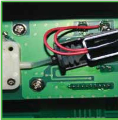
Self-replaceable sensor module allows for on-the-spot servicing. Used sensor modules can then be returned to us for recalibration and reuse.
